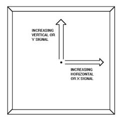
Two sensors must be installed 90° from each other to measure the entire amount of vibration in two planes (vertical and horizontal).
