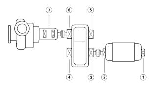
Distinguishing one bearing from another is an important consideration when installing or analyzing several bearings on a machine train. A common convention is to start numbering the bearings starting from the driver end. The choice of whether to use numbers or letters is immaterial; the sequence should increase as additional bearings are added to the diagram.
